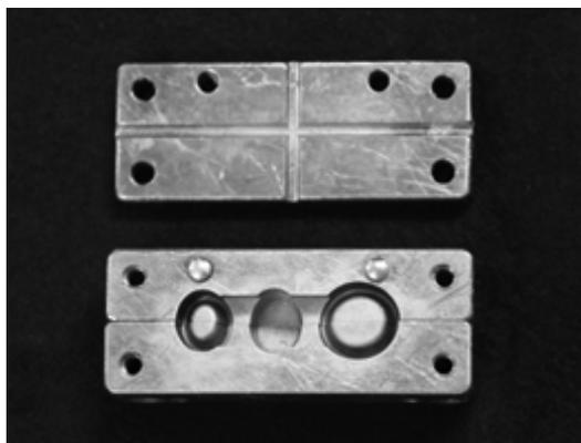
Figure 2 Fabricator designed and manufactured for production of PB
